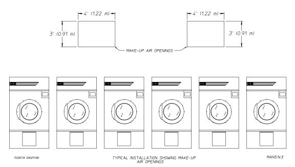
**IMPORTANT:** Make-up air *must be* provided from a source free of dry cleaning solvent fumes. Make-up air that is contaminated by dry cleaning solvent fumes will result in irreparable damage to the motors and other dryer components.
